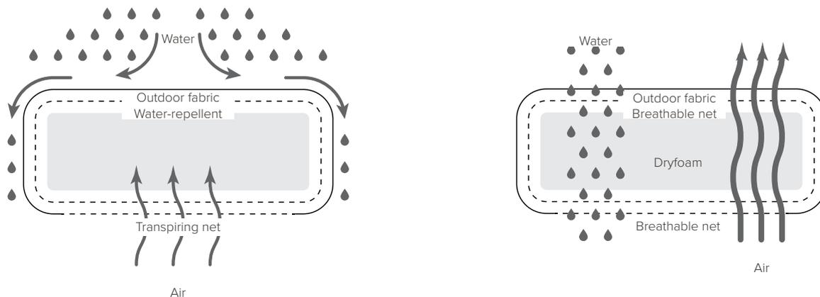
**water-repellent fillings** have a cover in a laminated, water-repellent polypropylene material which prevents water from penetrating. The thread used to stitch the seams swells when getting wet, preventing water from penetrating through the seams. On top of that, the seams are protected on the inside with an extra covering. If nevertheless water should penetrate, the material is breathable, letting moisture out to prevent moulding.
